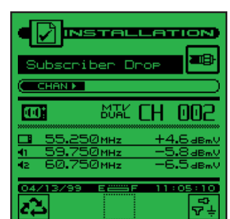
Pressing the “cycle” soft key provides a detailed view of what specific error is on the specific channel.
