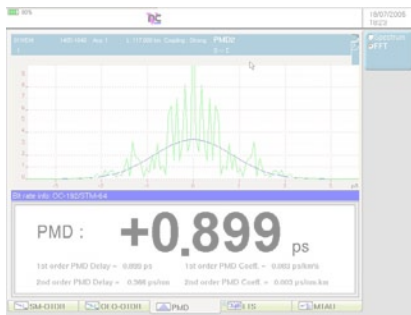
PMD test results with Pass/Fail analysis
