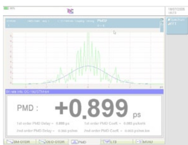
PMD test results showing the first order and second order PMD values
