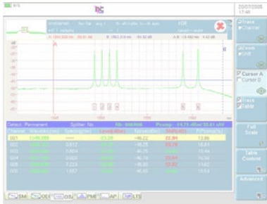
DWDM spectrum display with table of results
