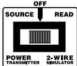
Move the slide switch to OFF to turn the 134-2 off. If AUTO-OFF is enabled, the 134-2 will turn itself off after 30 minutes of inactivity. Move the slide switch to OFF and to the right or left to turn the 134-2 back on.
