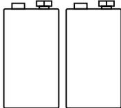
Low battery is indicated by BAT on the display. Approximately four hours of operation remain before the LCD blanks and POCKETCAL 134-2 shuts itself down. Turn the 134-2 off, loosen the captive screws securing the rear cover and lift off the cover from the top of the case. The two "9V" batteries are easily removed and replaced (alkaline supplied and recommended). Replace the bottom cover and tighten the screws.
