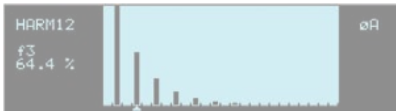
Harmonic waveform, Fund., 3 rd , 5 th , 7 th , 9 th , 11 th and 13 th .
